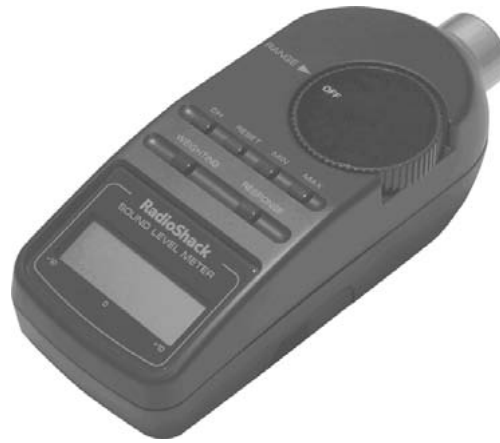
PHOTO 3: RS digital-display sound level meter.
